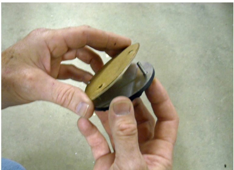
Place gasket over screws on new cover.
