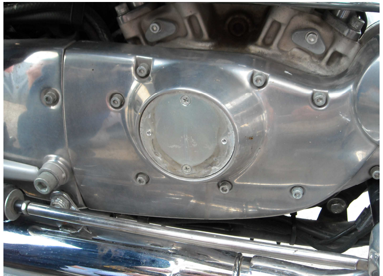
Unscrew top and bottom to remove inner cover.
