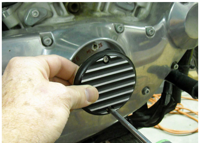
Screw new cover in place using Blue Loctite®.
