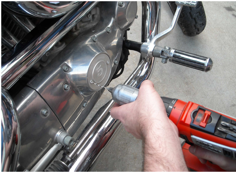
Drill out the outer cover rivets.
